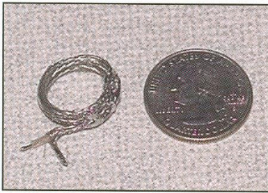
Photo 2A. This is a shorted 1/4\lambda loop made of RG174A with the outer insulation removed. This provides for a total delay of 1/2\lambda . Using the principle of skin effect the wave travels down the inside shield and then returns via the center conductor. The outside conductor is shorted at multiple points, thus behaving like one small loop. It showed promise, but its losses were too high.
