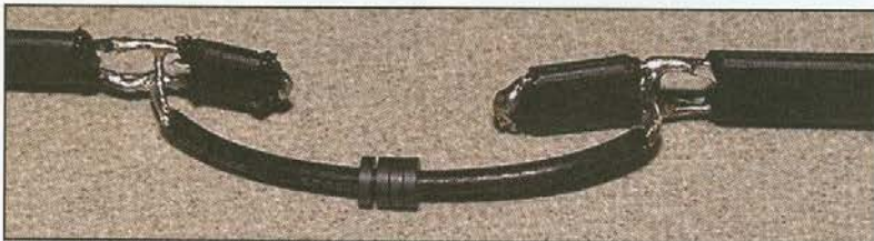
Photo 3. This is a close-up view of the interface between two J-pole pieces using RG174 coax. Four Amidon® Corp. FT-23-61 ferrites were inserted through the RG174 coax to minimize common mode currents.
